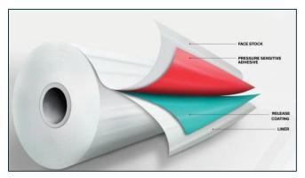
critical role in supporting the label during die-cutting, protecting its adhesive and providing a surface from which the selfadhesive label can be subsequently dispensed and applied. The silicone release coating itself is only a very thin coating on the surface of the base paper (typically only 1 micrometer in thickness, or 0.001 of a millimeter).
